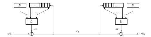
Fig. 1. Self-synchronizing stream encryption.
