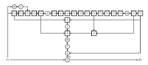
Fig. 2. Layout of SSS at the decryption side
