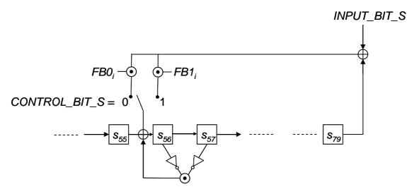
Figure 4: Clocking the *S* register
