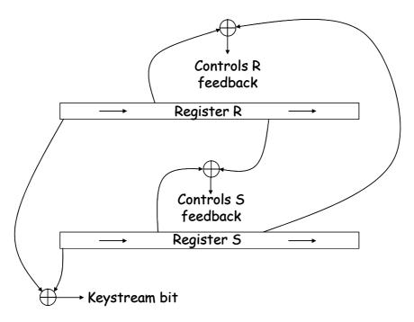
Figure 3: The variable clocking architecture
