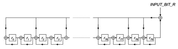
Figure 2: Clocking the *R* register with *CONTROL\_BIT\_R* = 1
