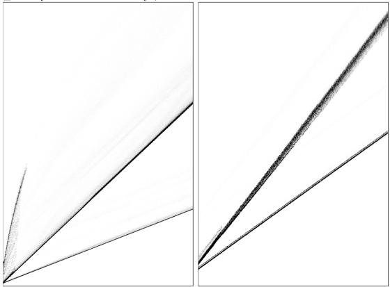
The sample graph on the right shows timings for the pypy-poly1305 system on a 2137MHz Intel Core 2 Duo (6f6) computer named katana. The spreading line shows variance in Pypy's stream-generation time, perhaps from cache-timing effects. Note also the large cost of handling small packets.
