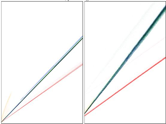
The graph on the right shows timings for the pypy-poly1305 system on the same computer. The wide spread of the dark line shows a considerable variance in Pypy's stream-generation time, perhaps because of cache-timing effects. Note also the relatively large cost of handling small packets.
