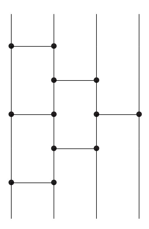
Positions of comparators in a sorting network are independent of the input. Naturally constant-time. Positions of comparators in a sorting network are independent of the input. Naturally constant-time.
