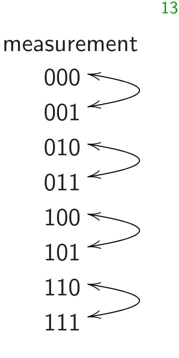
Operation on quantum state:  $NOT_0$ , swapping pairs. Operation after measurement: flipping bit 0 of result. Flip: output is not input.
