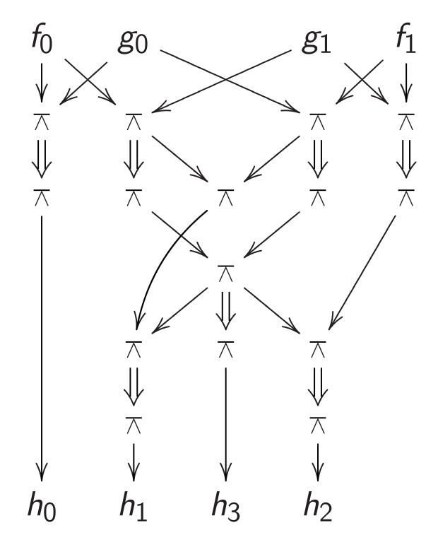
Gates  $\pi$ :  $a, b \mapsto 1 - ab$  computing product  $h_0 + 2h_1 + 4h_2 + 8h_3$  of integers  $f_0 + 2f_1$ ,  $g_0 + 2g_1$ .
