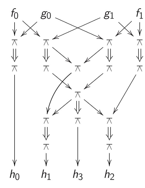
Gates  $\pi$ :  $a, b \mapsto 1 - ab$  comproduct  $h_0 + 2h_1 + 4h_2 + 8h_1$  of integers  $f_0 + 2f_1$ ,  $g_0 + 2g_2$
