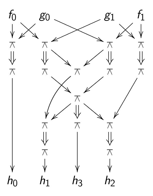
Gates  $\pi$ :  $a, b \mapsto 1 - ab$  computing product  $h_0 + 2h_1 + 4h_2 + 8h_3$  of integers  $f_0 + 2f_1$ ,  $g_0 + 2g_1$ .
