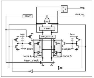
Figure 2: Entropy source for the Intel RNG (from [8])
