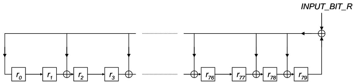
**Figure 1:** Clocking the  $R$  register with  $\text{CONTROL\_BIT\_R} = 0$
