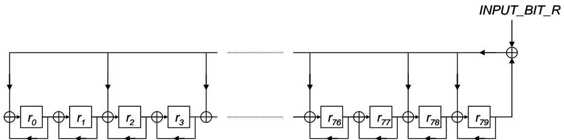
**Figure 2:** Clocking the  $R$  register with  $\text{CONTROL\_BIT\_R} = 1$
