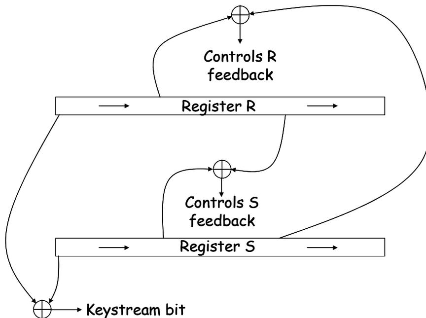
**Figure 3:** The variable clocking architecture
