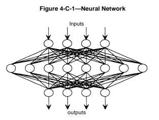
The circles represent processing elements that perform a weighted sum on their inputs and compute an output value that is then sent to the next layer of processing elements. SOURCE: OTA.
