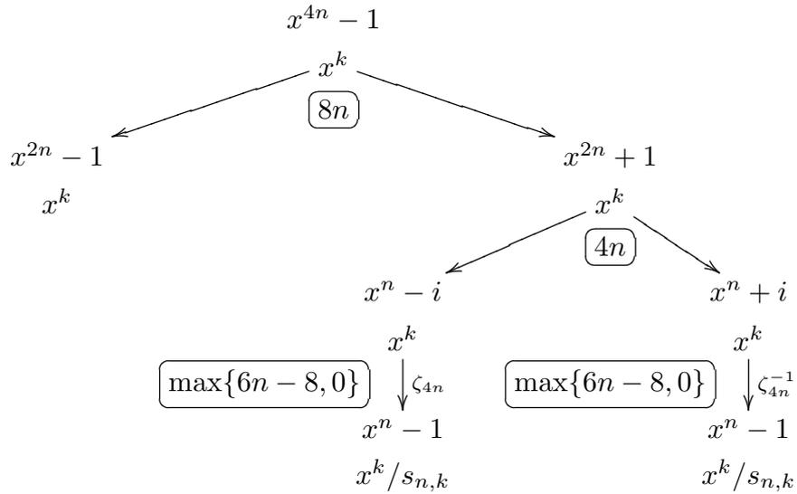
The coefficient of  $x^k$  in  $f \bmod x^n - i$  is now twisted by  $\zeta_{4n}^k s_{n,k}$ , costing 6 real operations except for the easy cases  $\zeta_{4n}^0 s_{n,0} = 1$  and  $\zeta_{4n}^{n/2} s_{n,n/2} = \sqrt{i}$ .
