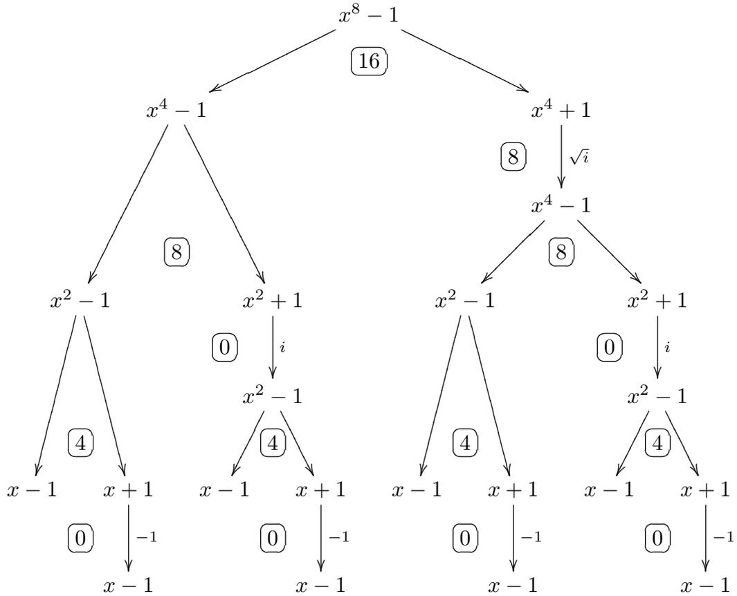
Note that the twisted FFT never has to consider moduli other than  $x^n \pm 1$ . The twisted FFT thus has a simpler recursive structure than the original FFT.
