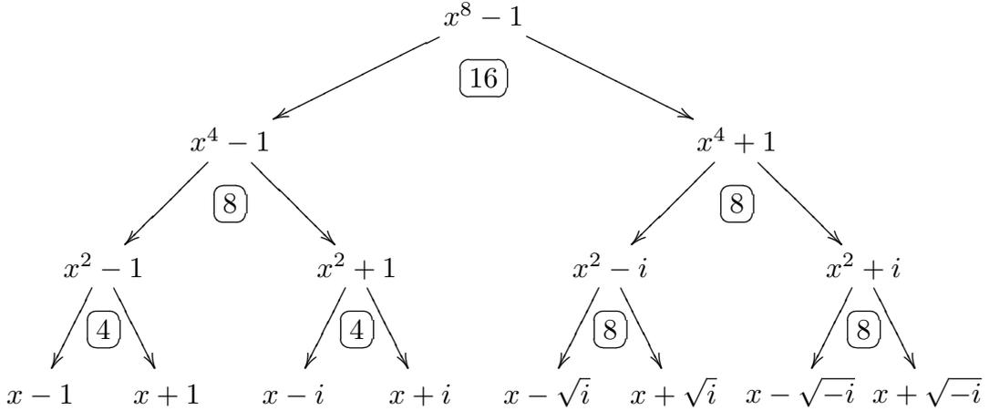
The final outputs  $f \bmod x - 1, f \bmod x + 1, f \bmod x - i, \dots$  are exactly the (permuted) DFT outputs  $f(1), f(-1), f(i), \dots$ , and this computation is exactly Gauss's original FFT. Note that the entire computation is naturally carried out in place, with contiguous inputs to each recursive step. One can further reduce the number of cache misses by merging (e.g.) the top two levels of recursion.
